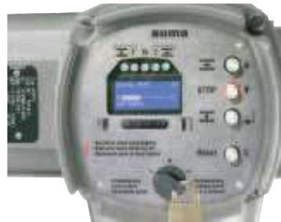
AUMATIC local controls with push buttons for operation and programming, selector switch, display with plain text display, indication lights and programming interface.
